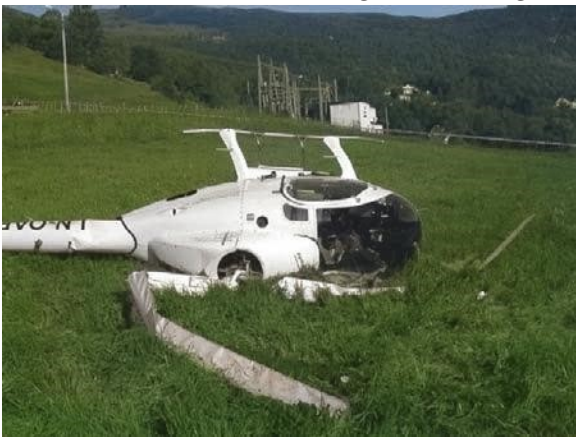
A hydraulic failure caused Sven to make an emergency landing and resulted in severe damage to the helicopter.
